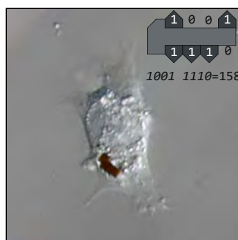
Fig. 2. Optical image a human macrophage with an intracellular silicon barcode and schematic view of the internalized code with its binary and decimal representation.
