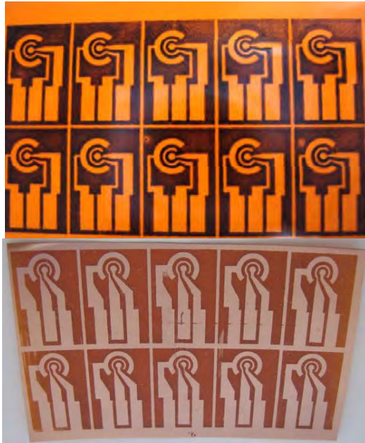
Two different steps of fabrication of micro-electrodes (illustrated for two different systems)
